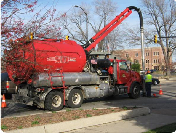
With the implementation of the City's Storm Water Utility and a storm sewer assessment study in hand, at risk areas were first cleaned then video taped. From the video, those sections of pipe and structures in a state of disrepair were identified. The project cleaned and video taped approximately 9000 lineal feet of storm pipe in seven locations and over 90 structures at a cost of \$28,356.80. The information will be used by the Engineering Division to prepare plans and specifications for the
