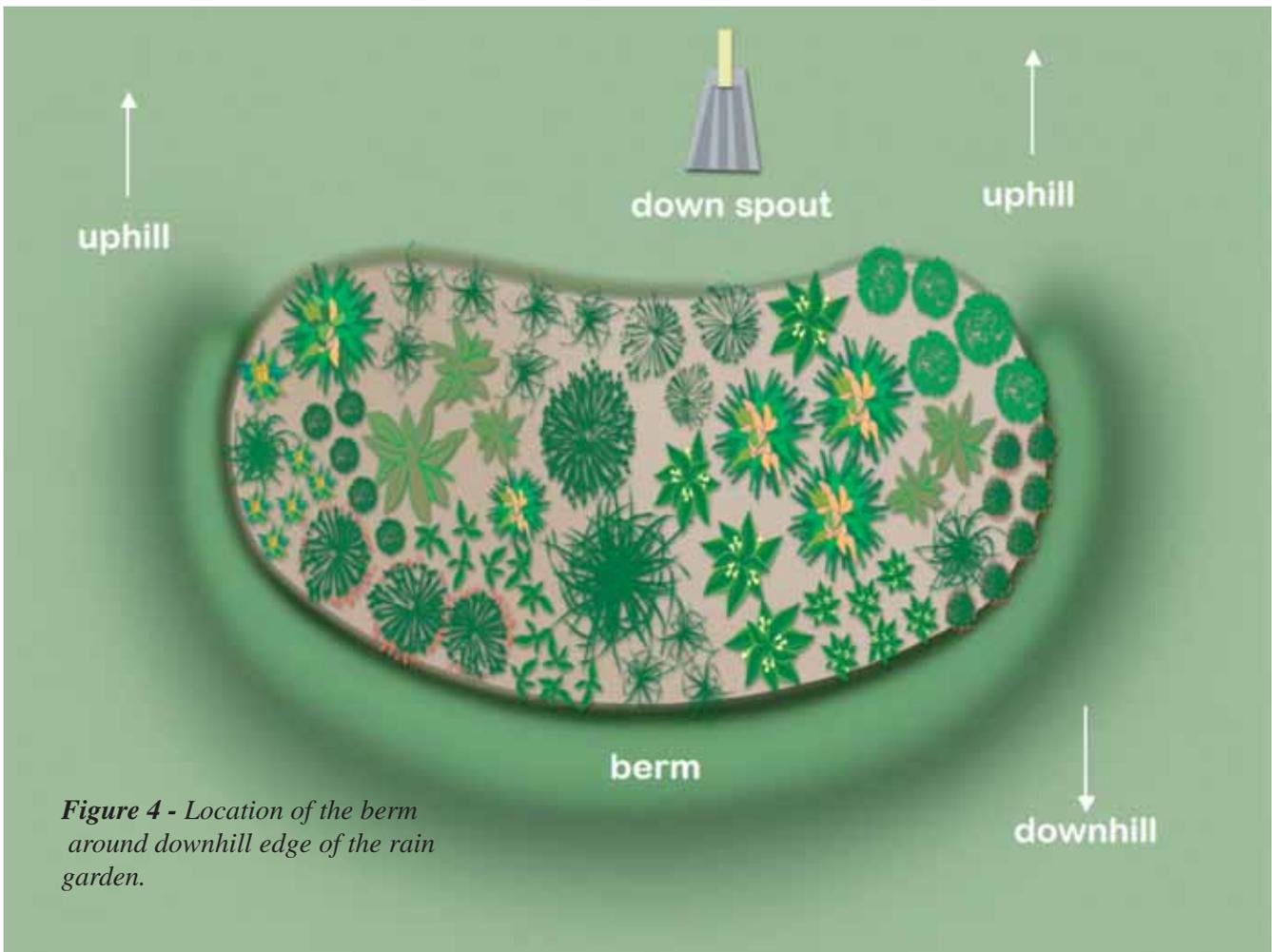
*Figure 4 - Location of the berm around downhill edge of the rain garden.*
